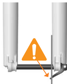
INCORRECTLY INSTALLED AXLE
