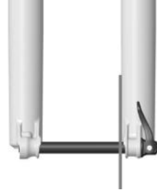
CORRECTLY INSTALLED AXLE
