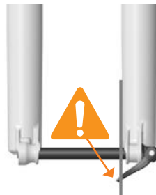
INCORRECTLY INSTALLED AXLE
