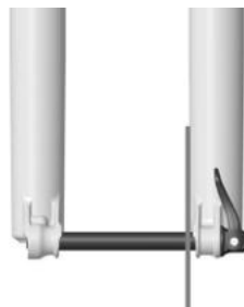
CORRECTLY INSTALLED AXLE
