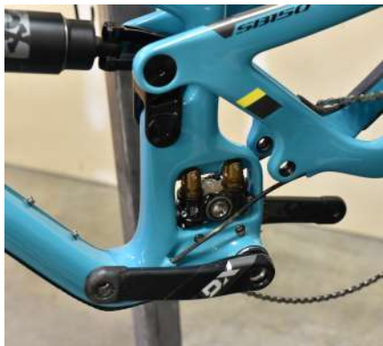
03. Rotate your swingarm upwards to access both grease zerk and expose the whole Switch Infinity link. With a clean rag and mild detergent, clean any mud, dust, or debris off the Switch Infinity Link.
