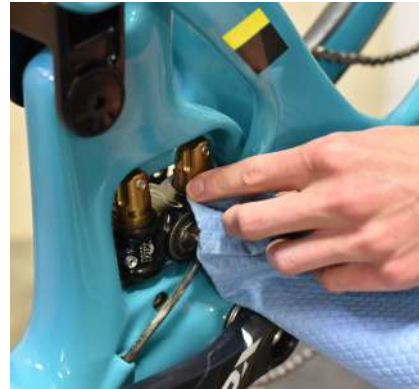
05. Wipe off any excess grease that was pushed out of the seals.
