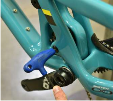
01. With a 5mm allen wrench, remove the main pivot Collet Wedge Bolt
