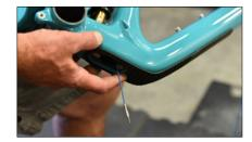
02 Drop a Park Tool Router tool down the seat tube until it exits the access port.
