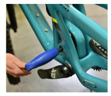
**02** With a 10mm allen wrench, remove the Main Pivot Collet Axle. The Collet Nut on the drive side can remain in the frame.
