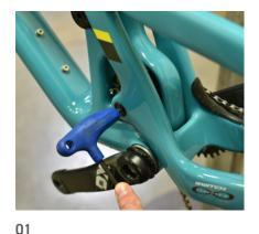
With a 5mm allen wrench, remove the main pivot Collet Wedge Bolt.
