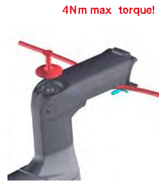
4Nm max torque! Install top cap and compression bolt
