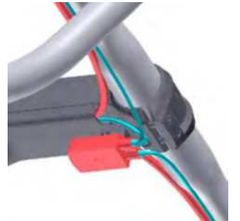
Install Di2 junction box (optional)
