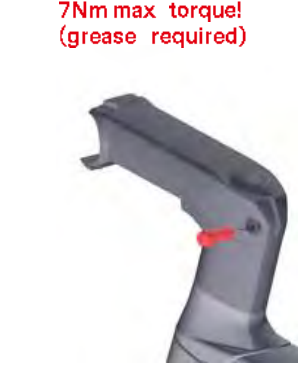
7Nm max torque! (grease required) Install stem steerer clamp bolt - grease required!
