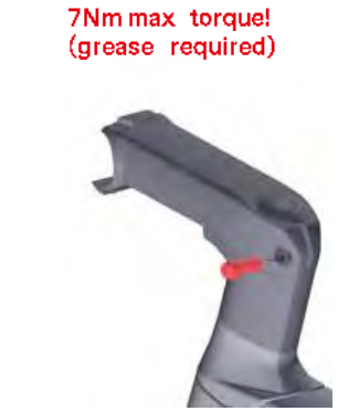
Install stem steerer clamp bolt - grease required!
