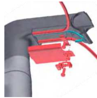
Install cable clamp, cable cover and Di2 junction box mount (optional)
