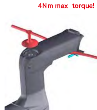
Install top cap and compression bolt
