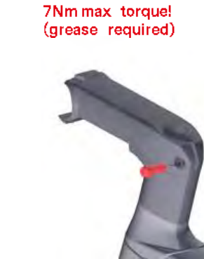
Install stem steerer clamp bolt - grease required!
