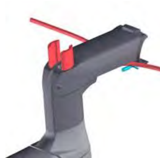
Install stem and steerer inserts
