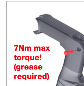
Install stem steerer clamp bolt - grease required!
