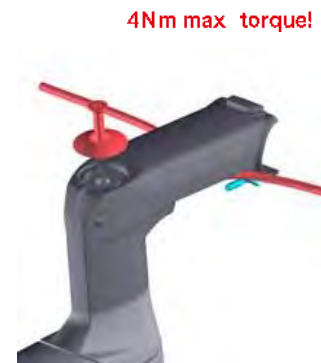
Install top cap and compression bolt
