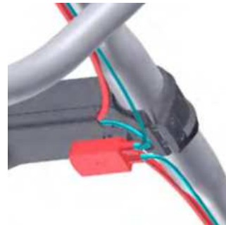
Install Di2 junction box (optional)
