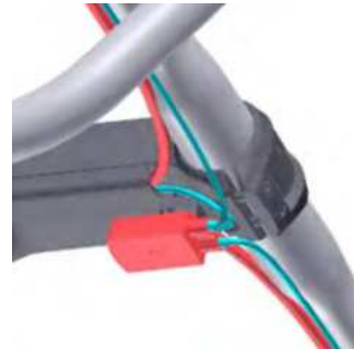
Install Di2 junction box (optional)
