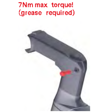
Install stem steerer clamp bolt - grease required!
