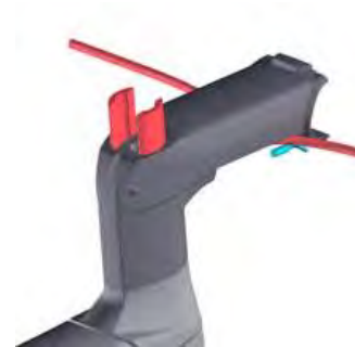
Install stem and steerer inserts
