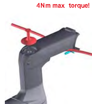
Install top cap and compression bolt
