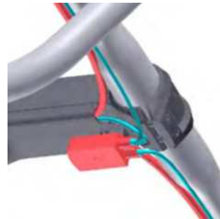
Install Di2 junction box (optional)
