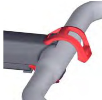
Install faceplate and faceplate cover make sure the top faceplate 'puzzle' clamp is securely engaged
