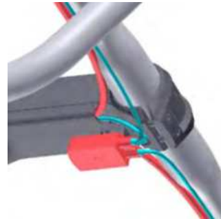
Install Di2 junction box (optional)
