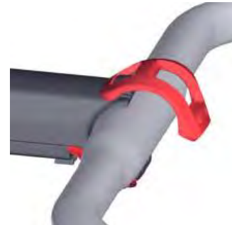
Install faceplate and faceplate cover make sure the top faceplate 'puzzle' clamp is securely engaged
