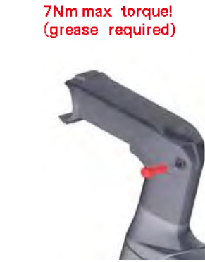
7Nm max torque! (grease required) Install stem steerer clamp bolt - grease required!
