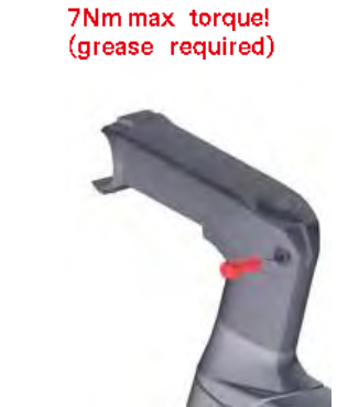
Install stem steerer clamp bolt - grease required!
