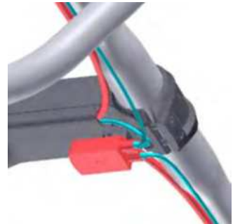
Install Di2 junction box (optional)
