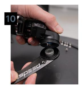
Align the OSPW RS System cage plate with the back of the derailleur, inserting the spring post into the low (L) tension setting on the cage (B). Do not worry about aligning the D shaped interface.
