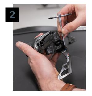
Remove the rear derailleur from the bike. Remove both pulley wheels and the back half of the pulley cage.
