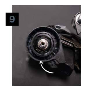
Mount the factory spring into the deraillur body. Be careful to place the spring post into the correct hole.
