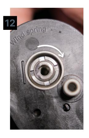
Take note of the mark you placed on the center post bolt in relation to the alignment mark on the OSPW RS System cage. Rotate the cage clockwise (looking at the nut and bolt interface) and ensure that the nut does not rotate or tighten. Rotate the cage until the alignment mark on the cage lines up with the mark placed on the threaded post.
