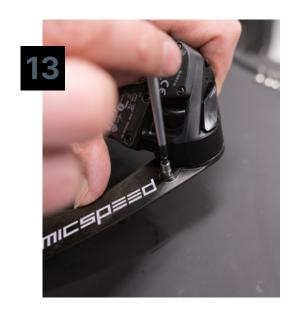
Rotate the OSPW RS System cage forward and install the rotation stop screw with a 2.5mm hex key. Tighten to a torque of 3.0Nm.
