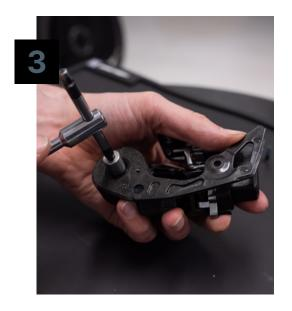
Hold the stock pulley cage (not just the derailleur) and loosen the main center nut with the CeramicSpeed special tool but do not completely remove the mounting nut. When the center nut is loose enough, allow the rotation stop screw to move past the stop point on the derailleur body to release the spring tension.
