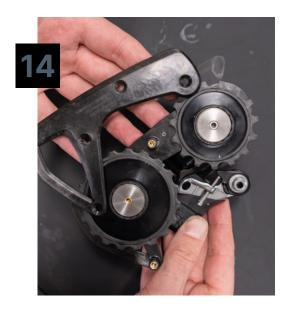
Install the 15 tooth pulley on the upper post and the 19 tooth pulley on the lower post of the OSPW RS cage, ensuring all four ADR shields are in place correctly and the pulleys are installed with the etching facing outward (toward the Front cage plate). Align the back cage plate and install the four 2.0mm cage bolts to a torque of 1.5Nm.
