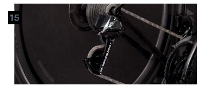
Install the derailleur onto the bike. Shift down to the bottom (smallest cog) and install the rear wheel. Measure a new chain following the guide below and check the upper and lower stop screws as well at the b-limit adjustment following the factory SRAM guidelines; 14mm for a 26T cog, 10mm for a 28T cog, and 5mm for a 33T or 36T cog.
