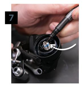
Mark the center screw end with a market to identify the flat surface of the D-shaped interface on the bottom of the center screw (A).
