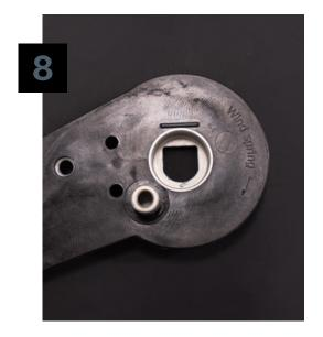
The CeramicSpeed cage is marked on the backside of the cage plate with a line to identify the flat side of the D-shaped interface.
