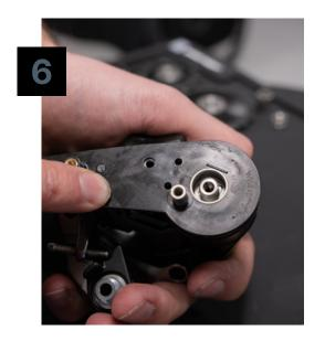
Using the CeramicSpeed front cage plate, rotate the D-shaped center post inside the derailleur counterclockwise until it stops. Remove the cage plate.
