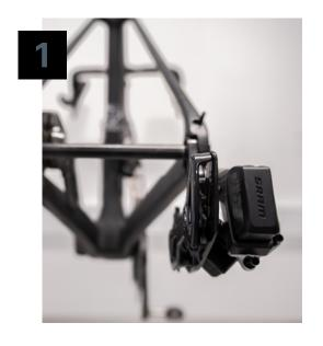
Begin with your bike mounted in a stand. Remove the chain. Remove the rear wheel. Then shift the derailleur up to the middle gear.
