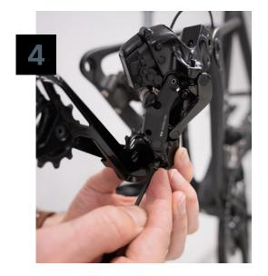
Shift the derailleur up so the cage will be able to rotate and not hit the derailleur body. For Ultegra 8150 or 105 7150, remove the rotation stop screw using a Philips screwdriver, and carefully allow the cage to unwind. For Dura Ace 9250, pull the cage by hand away from the derailleur body until the stop tower is free and carefully allow the pulley cage spring to unwind, releasing the spring tension. Your derailleur cage will appear to be upside down.
