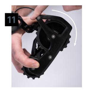
Hold the OSPW RS cage against the derailleur body and rotate counter-clockwise (first up and then to the back of the bike and downward) until you feel the ramped stop tower click past the stop point on the derailleur.
