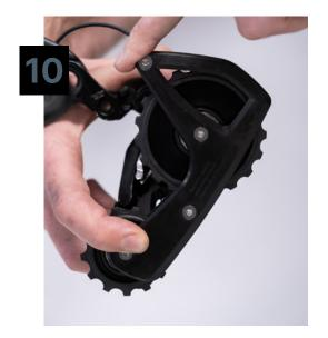
Rotate the derailleur body back, align the mounting post of the OSPW RS System to the back of the derailleur body with the cage pointing to the front of the bike. Align the tension spring and plastic spacer with the slot on the derailleur body and insert until the cage is flush to the derailleur. Ensure the OSPW RS cage rotates smoothly and the spring is properly secured.
