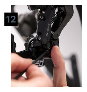
Secure the cage by reinstalling the original black T10 screw (removed at step 3). Installation torque is 1Nm. Your new OSPW RS System is now installed.
