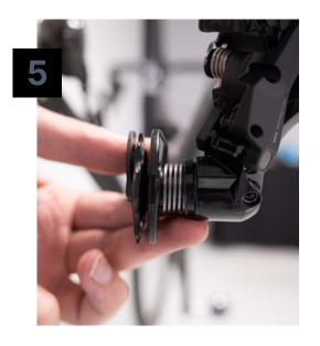
Slide out the original pulley cage and spring assembly, careful not to drop the pulley spring and plastic spacer.
