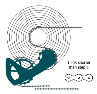
STEP 2: When tension is applied on the chain and the OSPW RS System appears to be aligned as the diagram on the left, the chain needs to be cut (1 link shorter than step 1) and connected by the required amount of links in order to achieve sufficient tension in this gear combination (always the small cog on the cassette).
