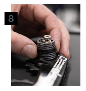
Note the four spring tension settings on the OSPW RS cage: from H (high) to L (low). The L tension setting will reduce both chain tension and friction, but will also result in slightly compromised shifting performance. The H tension setting will deliver the highest frictions levels but deliver the strongest chain retention for rougher roads or mixed surfaces.
