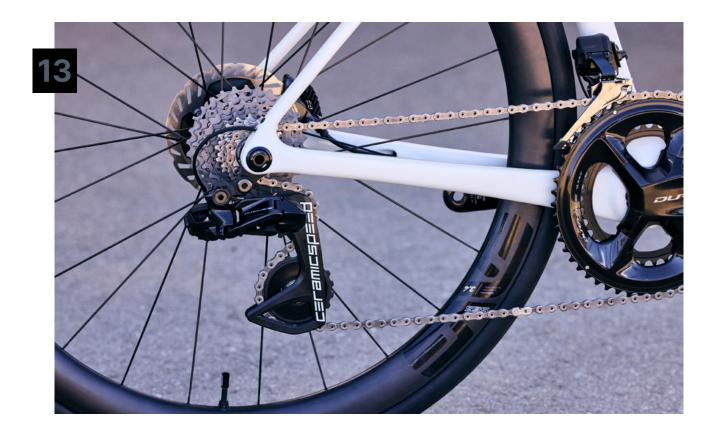
Shift the derailleur down to the bottom and install the rear wheel. Install a new chain according to the guide on the following page. Ensure the derailleur hanger is accurately aligned, check the upper and lower stops of the derailleur, and set the b-limit gap between 4-7mm at the largest cog and upper pulley. Adjust the Di2 trim for proper alignment between the cogs and pulley wheels. If in doubt, have a qualified mechanic make the final gear adjustments.
