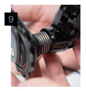
Select the spring tension hole second from 'L' (second lowest tension) and insert the hooked end of the spring completely. This may need to be pressed firmly. The plastic spacer will rest freely on the spring until aligned at the back of the derailleur body.
