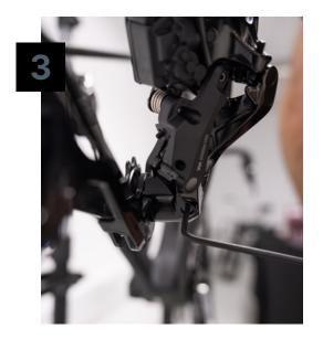
Locate the black mounting screw on the bottom of the derailleur body. Use a T10 Torx screwdriver to remove the black T10 mounting screw. Only half of the screw is threaded. Once the screw is about 1 cm out and the threads are not engaged, slide the screw the rest of the way out with your hand. Secure the cage in the derailleur body with your thumb.
