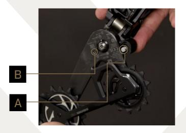
Once the spring tension is released, unscrew the main cage bolt (C) using the 3mm tamper bolt bit, to remove the cage from the clutch assembly and the derailleur housing. The clutch assembly remains inside the derailleur.
