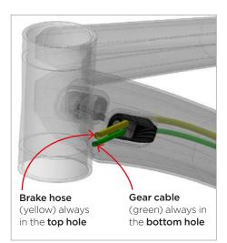
The MY20 Gambler offers internal cable routing, all these parts are available in one kit. There are two options for the headtube cable guides, blank and cabled, both come suppled in the kit.
