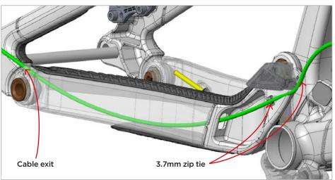
Ensure the all cables are clear of the shock in all suspension positions.
