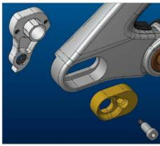
When fitting the rear axle ensure the groove in the head of the axle meets the dropout securing nut correctly.
