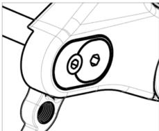
**Note:** it is normal for the rear derailleur and dropout to have movement and feel loose when the wheel is not fitted. Do not over tighten the securing bolt to compensate for this, once the wheel is fitted this movement will disappear.
