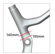
Riders must pay attention to the maximum/minimum seatpost insertion on the Gambler, there is only 15mm of up and down movement in the seatpost available, the rider must cut the seatpost to the required length and always pay attention not to exceed the recommended height.
