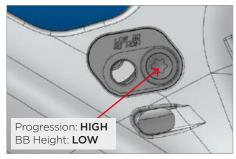
This flip chip and shock mounting bolts are available separately, lower shock bolt 10NM.
