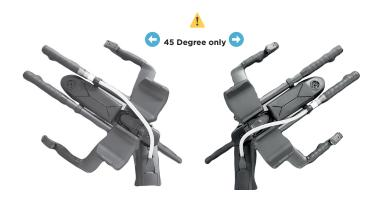
When riding, transporting, or storing your Plasma 6 take note of the limited turning rotation of the handlebars and fork.
