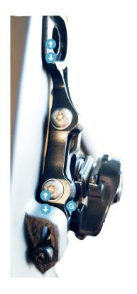
The left none drive side dropout can be moved inline with the right side by adjusting bolt **G** and sliding the complete unit backwards or forwards
