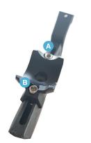
The seatpost bottle cage mount can be positioned to accommodate large drink bottles.
