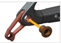
Before installing the new hanger first make sure the area is clean; insert the hanger.
