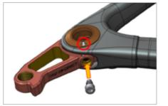
Make sure the location arrow is pointing to the lower bolt hole; insert the bolt (Max torque 1.5 N/M)
