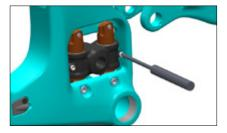
Using a needle-type grease gun, push new grease into the two Switch Infinity grease ports until you see fresh grease extruding from the shaft seals. Wipe off any excess grease that was pushed out of the seals.
