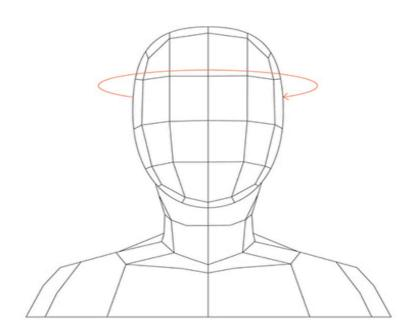
Helmet sizes are based on the circumference of your head. To determine the correct size, wrap a measuring tape around your head as shown in the diagram. Once you've determined your measurement, use the chart here to find your correct size.
