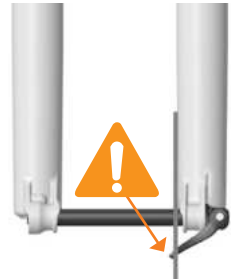
INCORRECTLY INSTALLED AXLE
