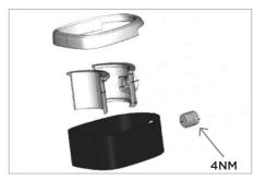
The seatpost clamp is specific to the Addict RC Disc.
