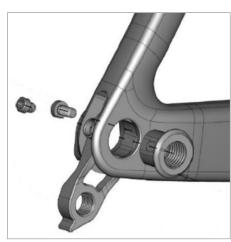
When amounting make sure the white arrow is aligned with the dropout rear bolt as below.
