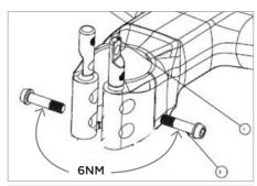
The Creston IC Stem will come as a complete kit as below, Creston IC SL will only be the fixation bolts.
