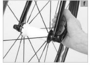
When continuing to close the lever the resistance you feel should increase significantly and towards the end even more strength is required to close the lever. Use the ball of your thumb while your fingers pull on an immovable part, such as the fork **(f, p. 33)** or a rear stay, but not on a brake disc or spoke, to push it in all the way.
