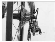
3. Check whether the chain still runs on the chainrings and the sprockets. If your SCOTT bike fell over to the chain side, verify the proper functioning of the gears. Ask somebody to lift your SCOTT bike by the saddle and carefully shift through all the gears. Pay particular attention when switching to the small gears, making sure the rear derailleur does not get too close to the spokes as the chain climbs onto the larger sprockets (c+d).
