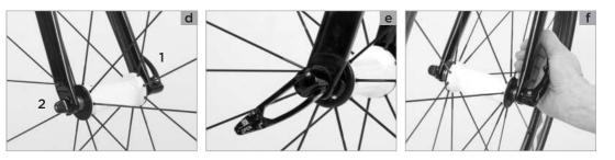
When continuing to close the lever the resistance you feel should increase significantly and towards the end even more strength is required to close the lever. Use the ball of your thumb while your fingers pull on an immovable part, such as the fork **(f, p. 33)** or a rear stay, but not on a brake disc or spoke, to push it in all the way.
