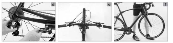
6. Finally, take a good look at the whole SCOTT bike to detect any deformations, colour changes or cracks. Ride back very carefully by taking the shortest route possible.
