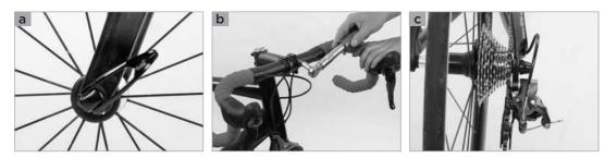
3. Check whether the chain still runs on the chainrings and the sprockets. If your SCOTT bike fell over to the chain side, verify the proper functioning of the gears. Ask somebody to lift your SCOTT bike by the saddle and carefully shift through all the gears. Pay particular attention when switching to the small gears, making sure the rear derailleur does not get too close to the spokes as the chain climbs onto the larger sprockets (**c+d**).
