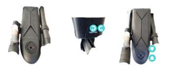
The Nutrition Box between the handlebar extensions can be tilt downwards so you can attached a larger GPS unit.
