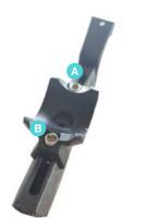
The seatpost bottle cage mount can be positioned to accommodate large drink bottles.
