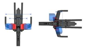
The width, forward and backward adjustment of the pad can be adjusted.
