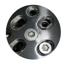
⚠ Tighten only two bolts to 5 Nm, with the addition of Blue Loctite.
