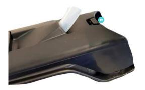
The Top Tube Hydration Bottle can be released from the frame by pressing • gently.
