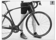
6. Finally, take a good look at the whole SCOTT bike to detect any deformations, colour changes or cracks. Ride back very carefully by taking the shortest route possible.
