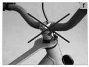
5 | 20 ENGLISH OWNER'S MANUAL | KIDS' TOY BICYCLE KIDS' TOY BICYCLE | OWNER'S MANUAL ENGLISH 21 | 5 Now you can move the handlebar/stem-unit up and down as a whole. Be sure not to pull out the stem too far. The mark on the stem (end. min. max. stop. limit or the like) should always remain within the tube (a). Setting the stem to a lower position can only add to your safety!
