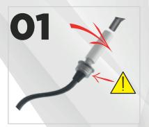
Attach the upper shock pump head to the shock valve, making sure the lower part of the pump head stays in the lower position.
