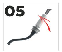
Unscrew the upper shock pump head from the shock valve.
