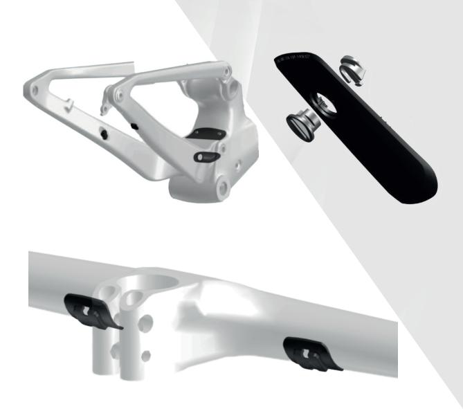
Please be aware that the maximum bolt length for the bottle cage on the seat tube is 10mm. The rivet nuts have closed ends, and using a longer bolt may result in damage to the frame.
