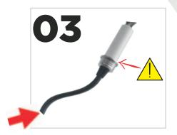
Make sure there is no gap between the two shock pump heads. Then pump the air to the required pressure.
