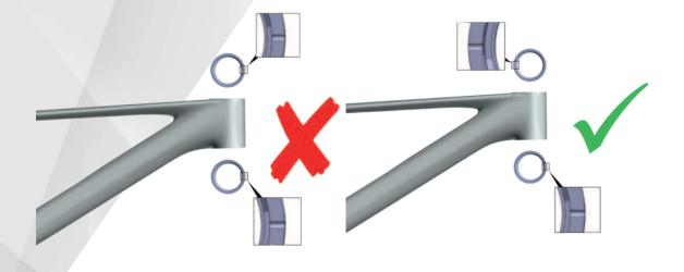
The headset assembly must follow the below no matter which bar/stem system is being used.
