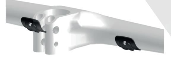
Please be aware that the maximum bolt length for the bottle cage on the seat tube is 10mm. The rivet nuts have closed ends, and using a longer bolt may result in damage to the frame.
