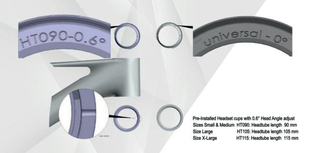
For  $0.6^{\circ}$  this can be installed at  $+ \text{ or } - \text{ but it is essential that the angle indication markers on the headset are set opposite to each other, top facing forward and bottom facing backwards (or vice versa).$
