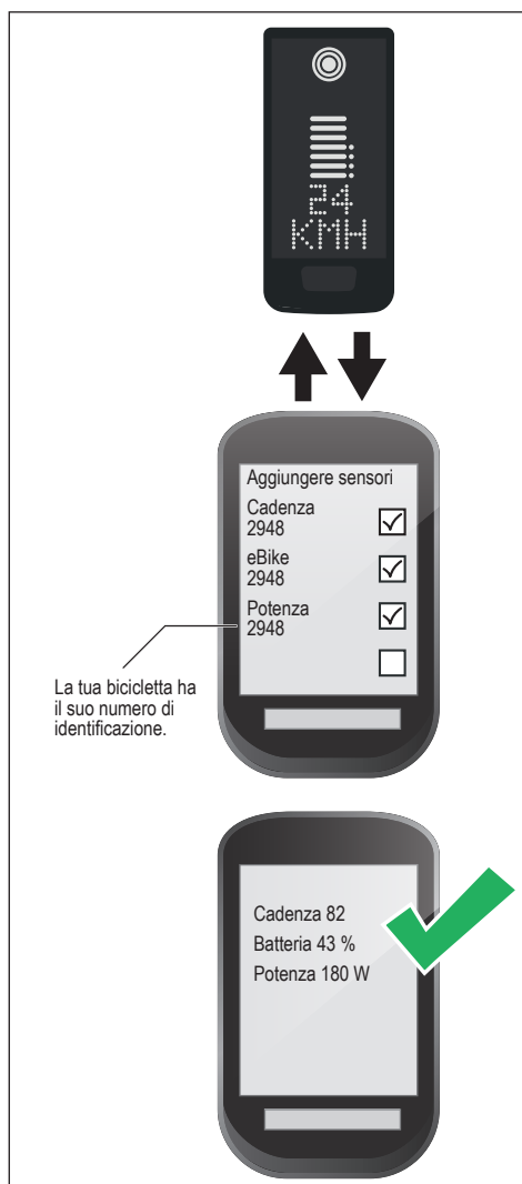
Fig. 8: Connessione e-Bike al cicocomputer
