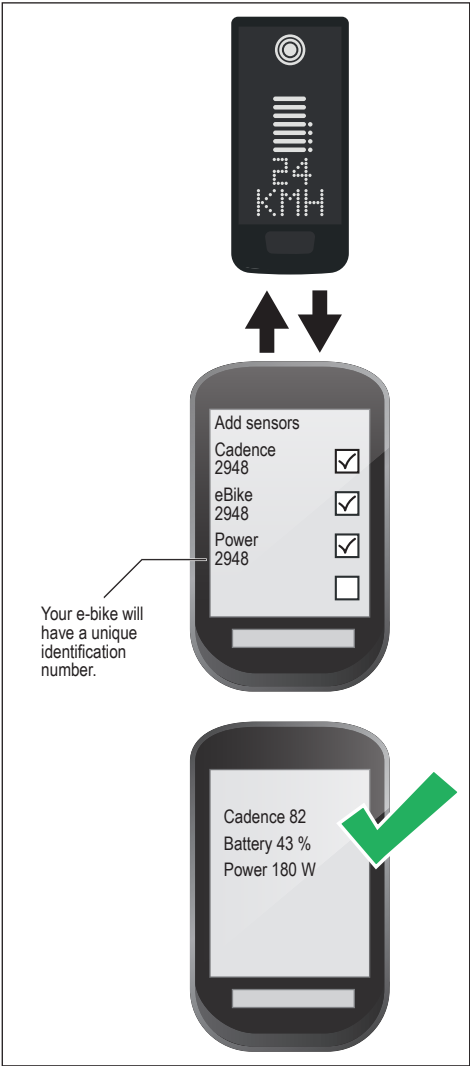
Fig. 8: Connection e-bike to bicycle computer
