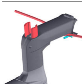
Install stem and steerer inserts
