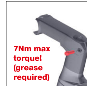
Install stem steerer clamp bolt - grease required!
