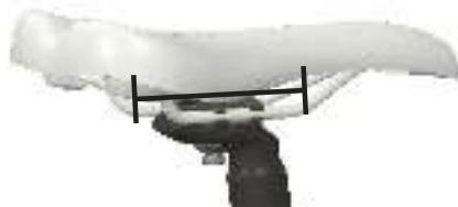
STRAIGHT SECTION OF THE SEAT RAILS
