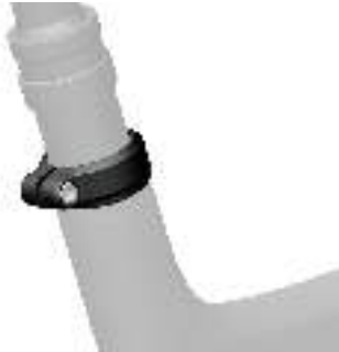
FIXED-BOLT SEATPOST COLLAR
