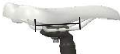
STRAIGHT SECTION OF THE SEAT RAILS
