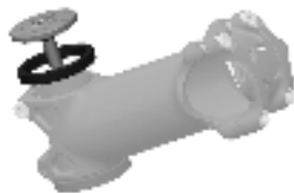
STEM, SPACER, AND TOP CAP
