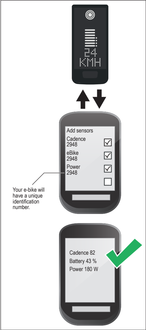
Fig. 8: Connection e-bike to bicycle computer
