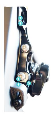
The left none drive side dropout can be moved inline with the right side by adjusting bolt **G** and sliding the complete unit backwards or forwards
