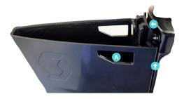
The Storage Box behind the seat tube can be accessed by pressing points (a) on the lid both sides (lid not pictured).
